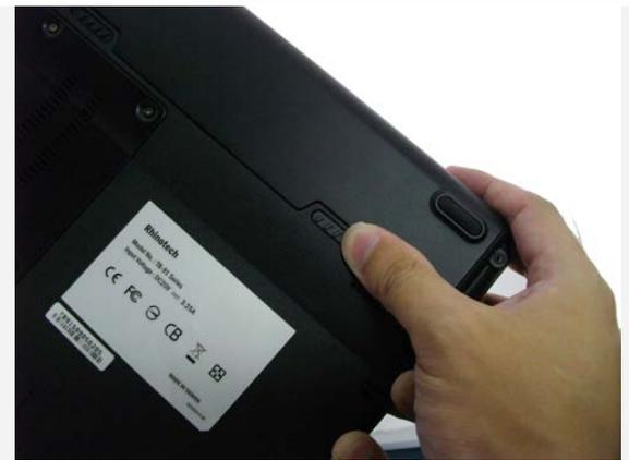
**Step 3 Ensure battery is seated correctly**
