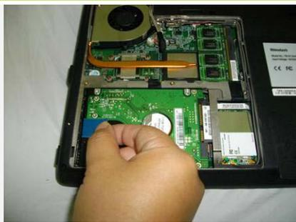
**Step 2 Fit new drive and insert the packing rubber**
