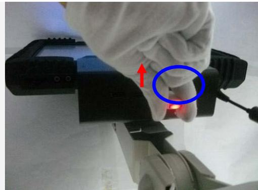
Check USB socket at the bottom of the cradle
