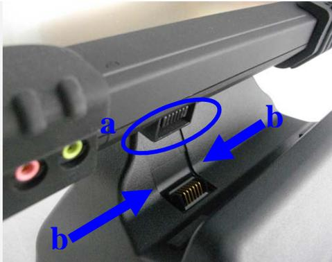
Ensure that docking port (a) at the rear of the tablet is aligned with the inset slot (b) on the docking station.
