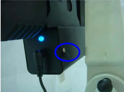
Fasten screw to fix the hook to cradle
